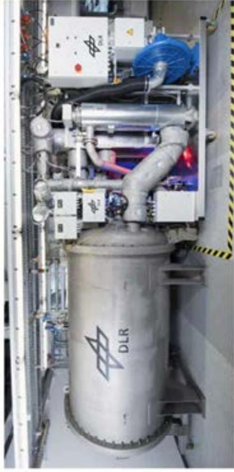
SOFC hybrid test rig after the assembly
