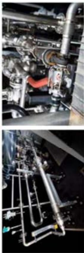
Set-up of the MGT hybrid test rig (left) and detail of the power module and combustion chamber in the test rig (right) before insulation
